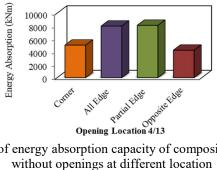
Fig. 12. Comparison of energy absorption capacity of composite space truss with and without openings at different location
