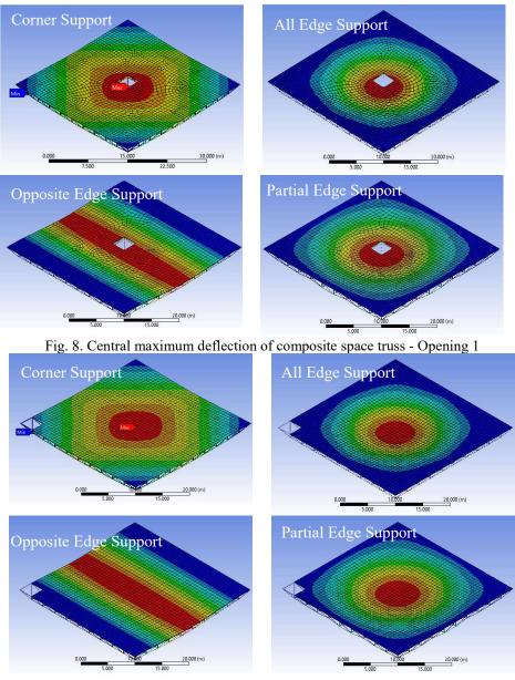
Fig. 9. Central maximum deflection of composite space truss - Opening 11/25
