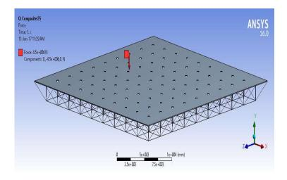
Fig. 4. Model of the composite space truss
