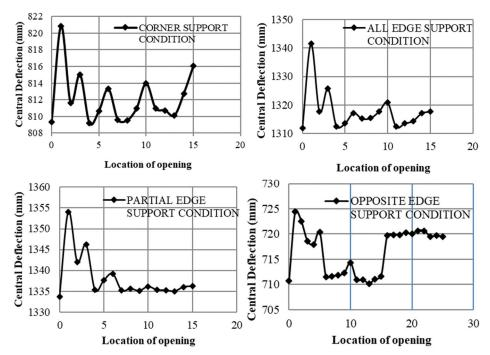
Fig. 5. Comparison between the central deflections of the composite space truss for varying location of openings
